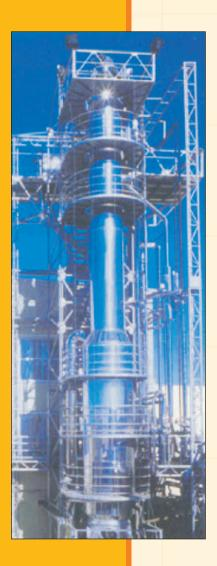
Multistage Deodorisers are in stainless steel construction with heating and cooling oil under vacuum. The Deodorisers have special sparge steam nozzles and mammoth pumps for uniform and aggressive mixing of steam and oil. Heating arrangement both with thermic fluid heating system or with high pressure steam thermosyphon are available. Adequate retention time is provided for light colours. Refined oils produced have high retention of tocopherols for stability of refined oils produced.
